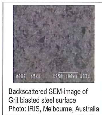
SEM-Image of grit blasted steel surface with embedded grit.
